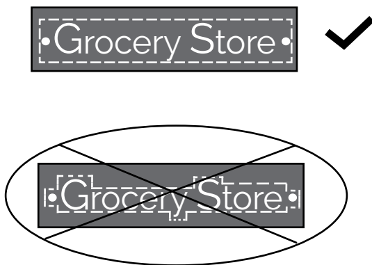
Figure 9.1-1 Calculating Sign Face Area.
