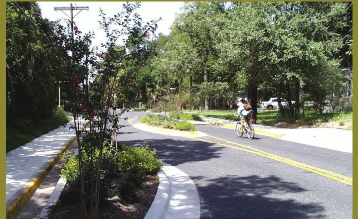
Chicane, Source: nacto.org/publication/urban-street-design-guide/street-design-elements/curb-extensions/chicane/
