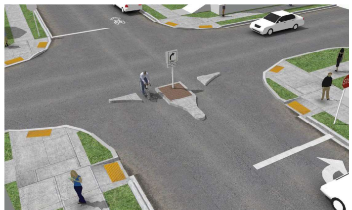
T-Intersection Diverter. Source: NACTO
