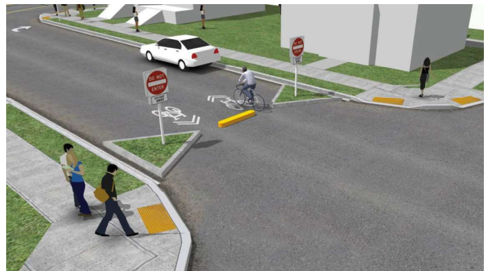
Full Roadway Diverter. Source: NACTO
